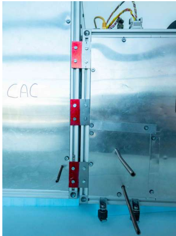
Figure 108: Fast Recovery Interfaces detail, boxes attachment.
