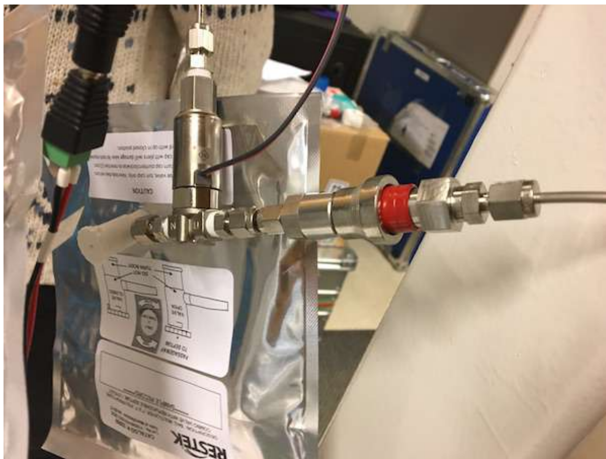
Figure 162: 1 L Sampling Bag With SMC Valve Attached to It. The Valve is at One of the Ends of the System so a Quick Connector is Connecting it to the Tube That Goes to the Nitrogen Bottle/Vacuum Pump.
