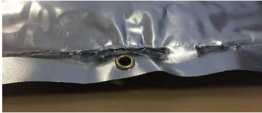
Figure 156: Photo Showing the Extent of Damage on the Front of the Bag Due to Bursting.
