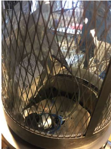
Figure 154: Photo Showing the Pump and Sampling Bag in the Vacuum Chamber During the Test.
