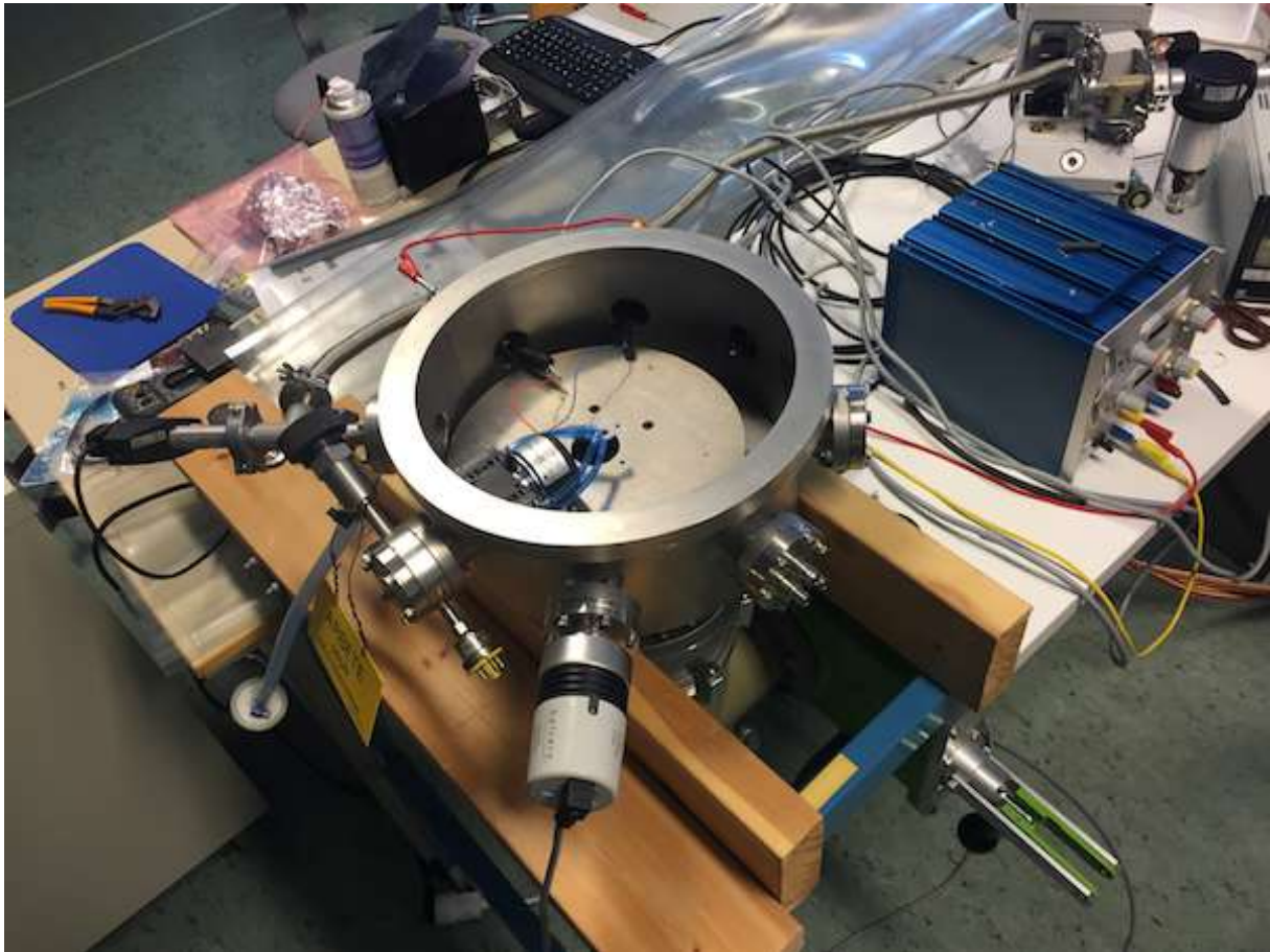
Figure 153: Photo Showing the Set-up of the Vacuum Chamber, Power Supply and Vacuum Pump.
