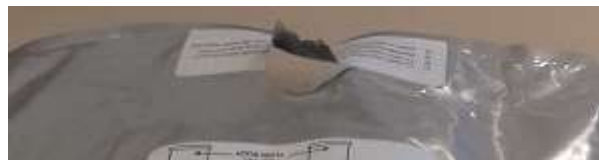
Figure 159: Photo Showing Where the Bag Ripped Around the Valve.
