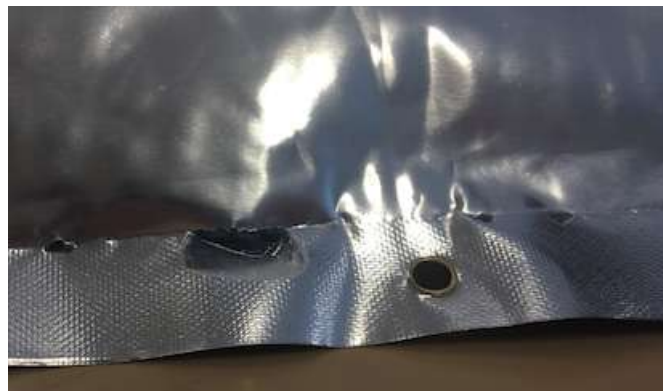
Figure 157: Photo Showing the Extent of Damage on the Back of the Bag Due to Bursting.
