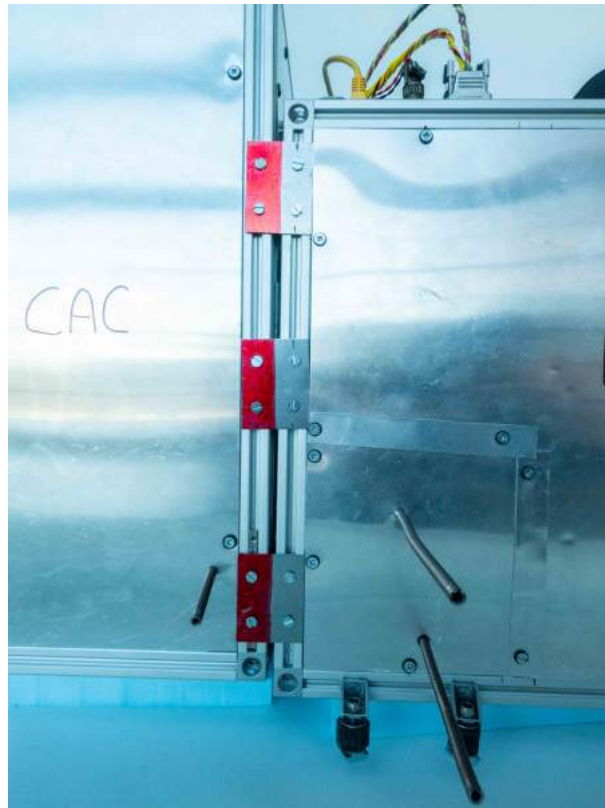
Figure 109: Fast Recovery Interfaces detail, boxes attachment.
