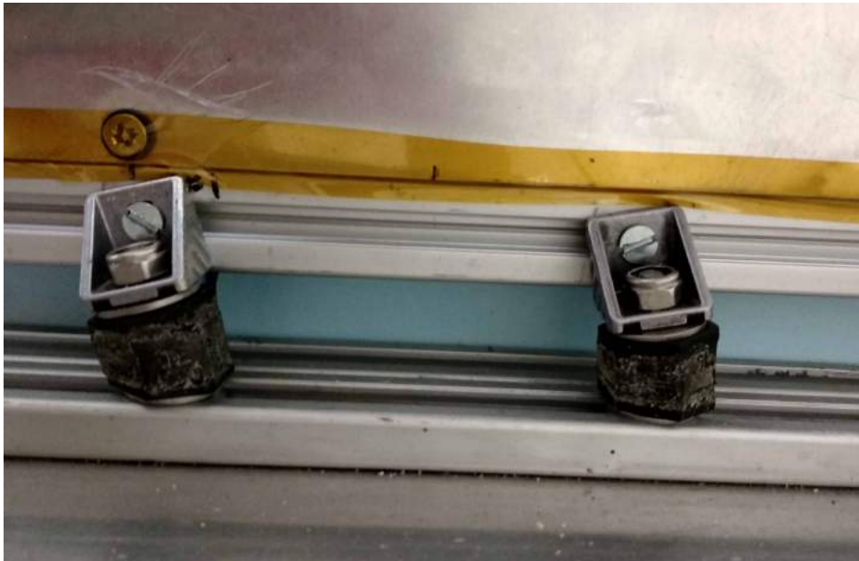
Figure 62: Position of the bumpers after landing.
