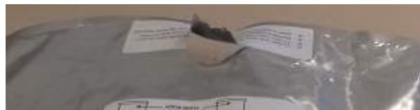
Figure 160: Photo Showing Where the Bag Ripped Around the Valve.
