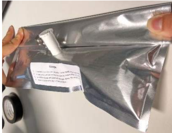
Figure 174: Picture Showing the Air Remaining in the Bag After Returning to Sea Level Pressure.
