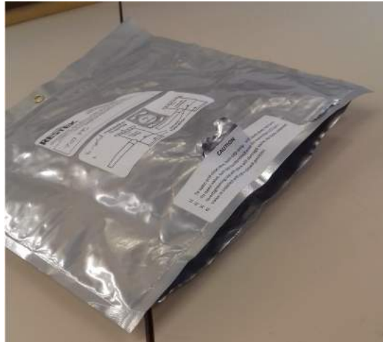
Figure 159: Photo Showing the Damage Sustained to the Bottom of the Bag After Bursting Due to Continuous Pumping.
