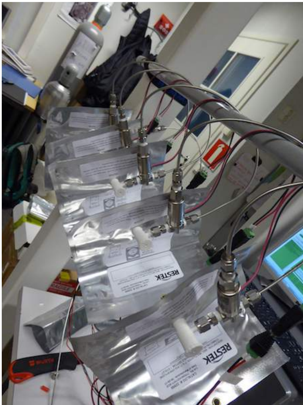
Figure 164: Sampling Bags System Connected in Series.
