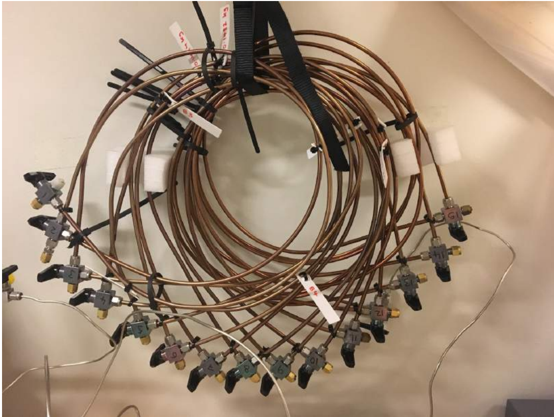
Figure 61: CAC Sampler with 15 Different Stages.
