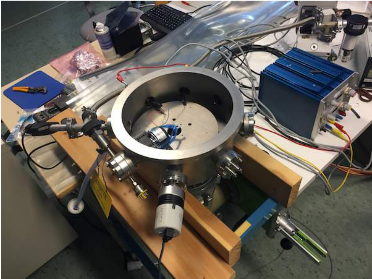
Figure 154: Photo Showing the Set-up of the Vacuum Chamber, Power Supply and Vacuum Pump.
