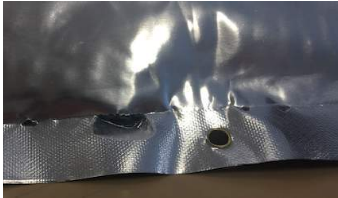
Figure 158: Photo Showing the Extent of Damage on the Back of the Bag Due to Bursting.
