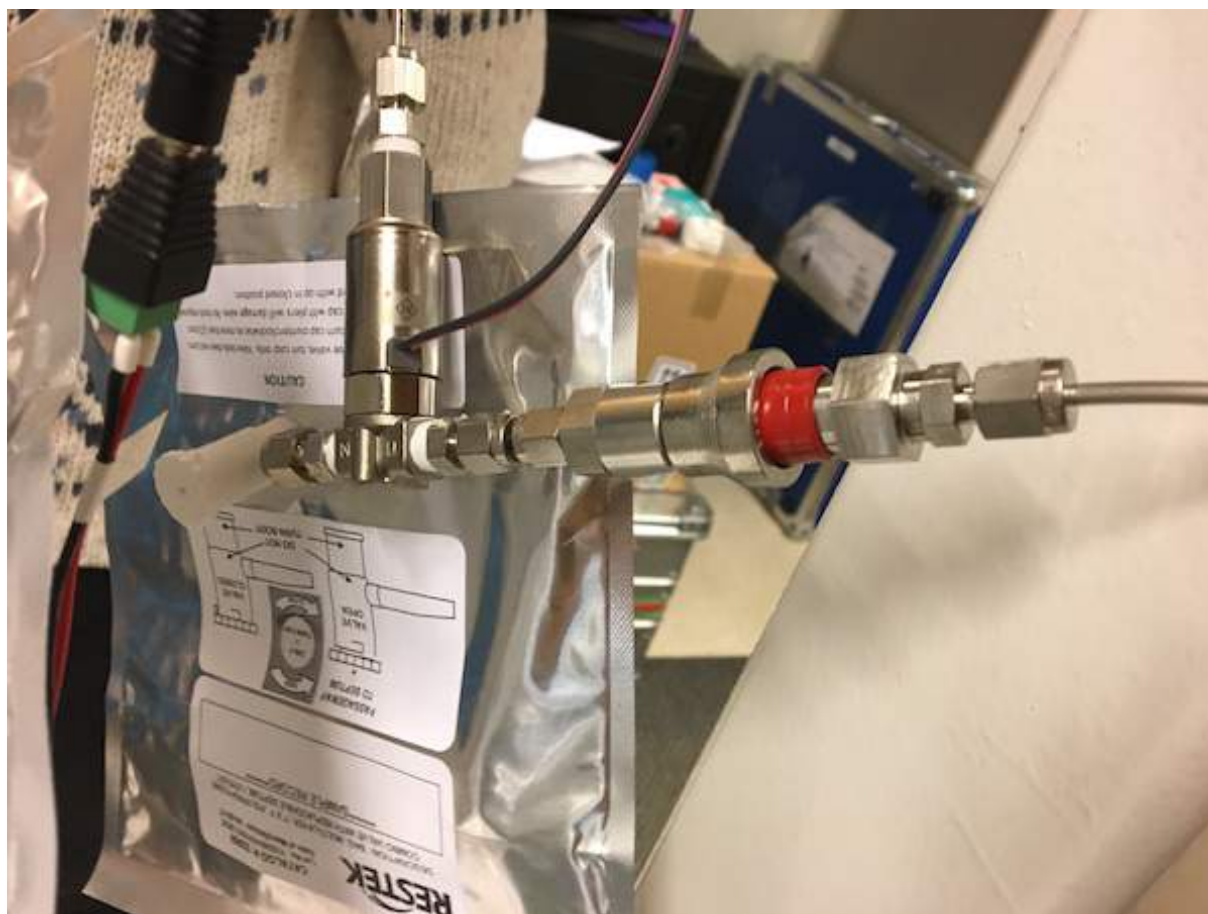
Figure 163: 1 L Sampling Bag With SMC Valve Attached to It. The Valve is at One of the Ends of the System so a Quick Connector is Connecting it to the Tube That Goes to the Nitrogen Bottle/Vacuum Pump.
