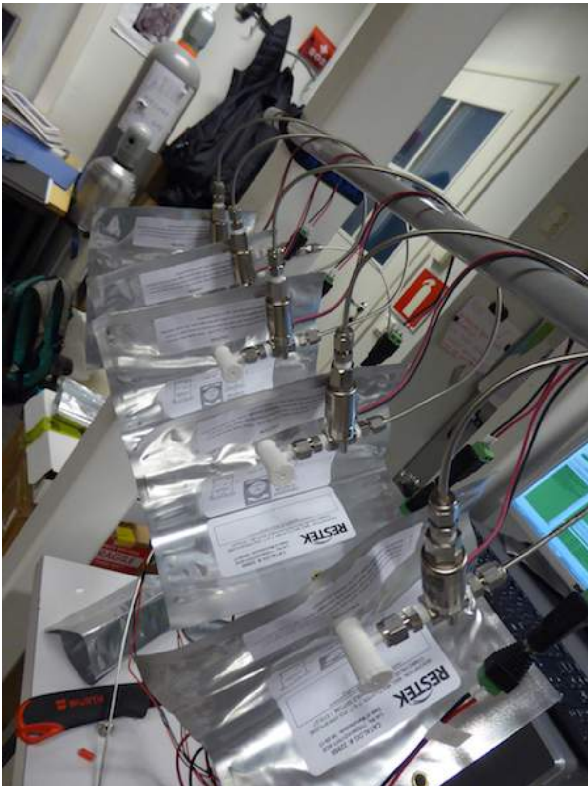
Figure 164: Sampling Bags System Connected in Series.
