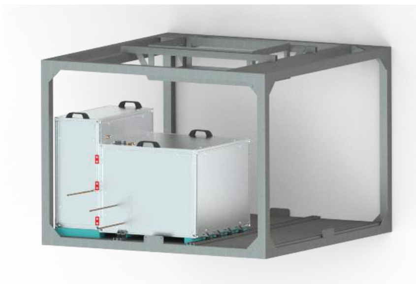
Figure 50: Example of Experiment Box Accommodation Inside the Gondola.
