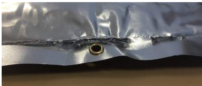
Figure 157: Photo Showing the Extent of Damage on the Front of the Bag Due to Bursting.
