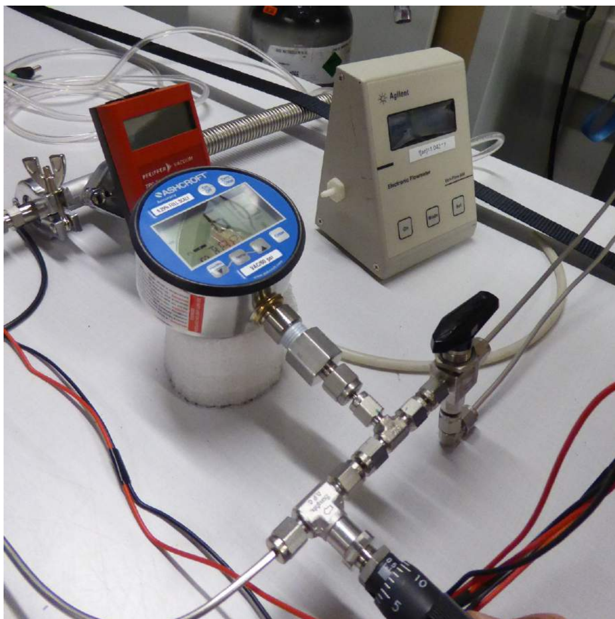
Figure 166: Valve that Controls Filling/Vacuum in of the Sampling Bags. Pressure Sensor, Flow-metre and Needle Valve.
