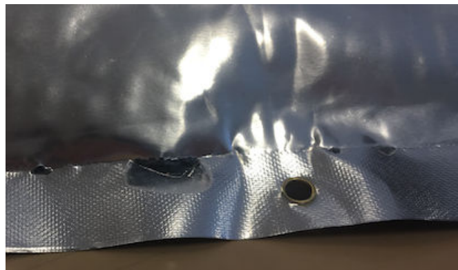
Figure 143: Photo Showing the Extent of Damage on the Back of the Bag Due to Bursting.
