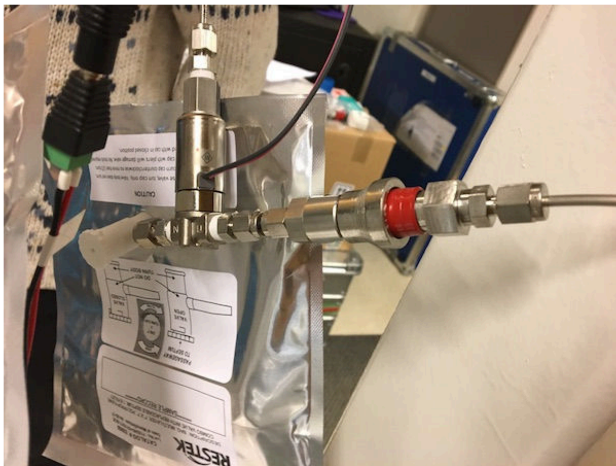
Figure 148: 1 L Sampling Bag With SMC Valve Attached to It. The Valve is at One of the Ends of the System so a Quick Connector is Connecting it to the Tube That Goes to the Nitrogen Bottle/Vacuum Pump.
