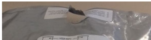
Figure 145: Photo Showing Where the Bag Ripped Around the Valve.
