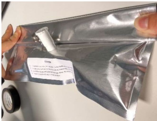
Figure 159: Picture Showing the Air Remaining in the Bag After Returning to Sea Level Pressure.
