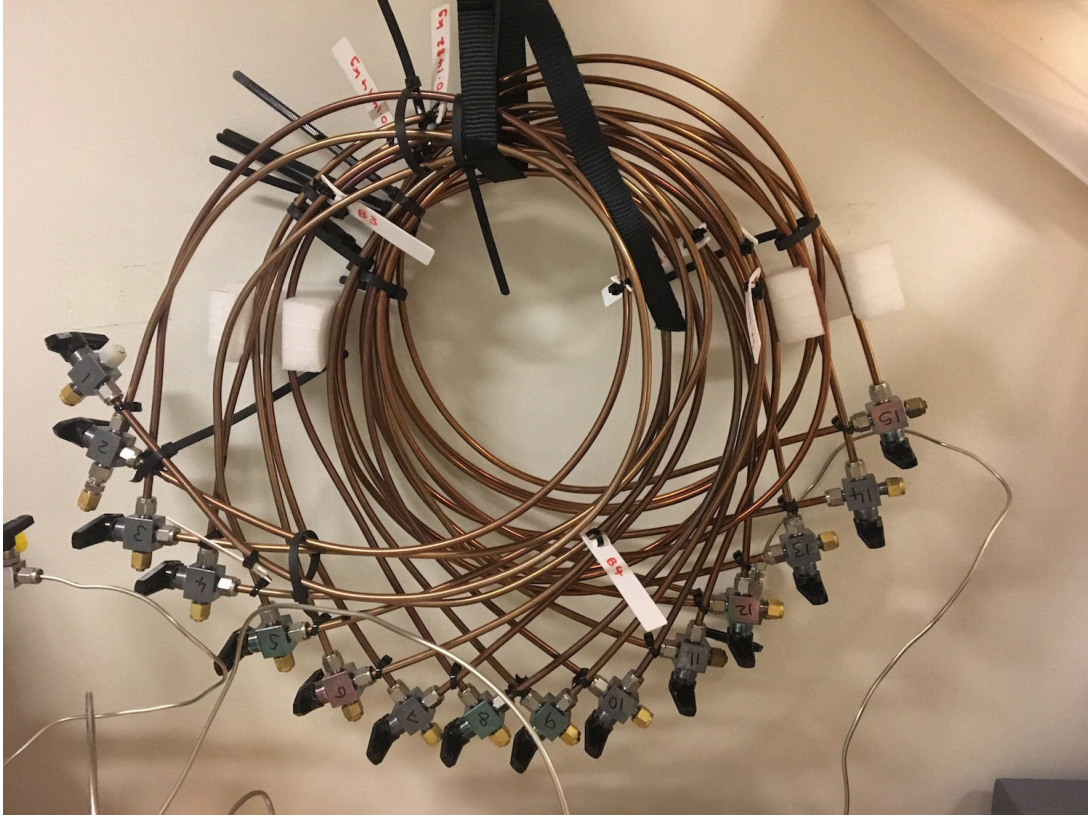
Figure 56: CAC Sampler with 15 Different Stages.
