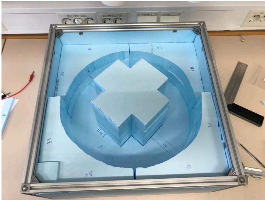
Picture 2: Frame for Air Coil including insulation material
