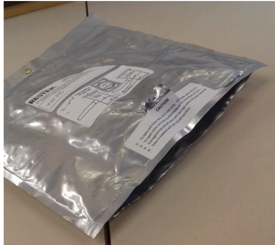
Figure 144: Photo Showing the Damage Sustained to the Bottom of the Bag After Bursting Due to Continuous Pumping.
