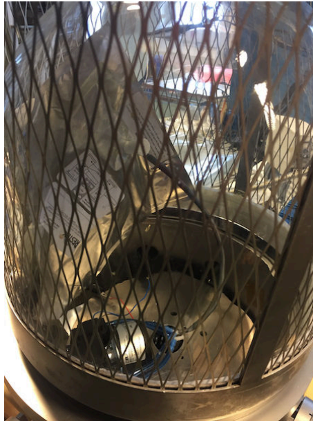
Figure 140: Photo Showing the Pump and Sampling Bag in the Vacuum Chamber During the Test.
