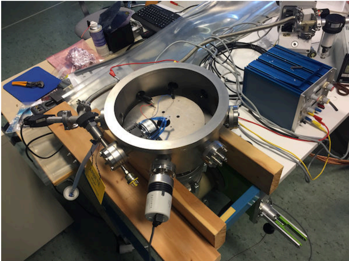
Figure 139: Photo Showing the Set-up of the Vacuum Chamber, Power Supply and Vacuum Pump.
